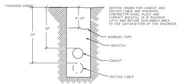
CONDUIT, DUCTED CABLE AND WARNING TAPE TRENCH
